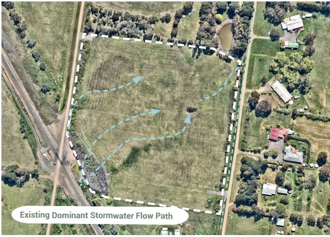
figure 3. Existing Stormwater Flow Path
